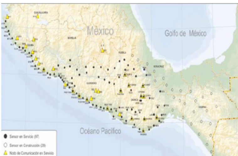
Image 2 Distribution of sensing stations used in the Mexican Seismic Alert System (Image source: CIRES, Mexico)
