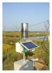
Figure 39 Automatic Weather Station and Automatic Rain Gauge network are one of the primary requirement for a robust Early Warning System for the agriculture sector (Source: Department of agriculture, Government of Bihar, India and ADPC)
