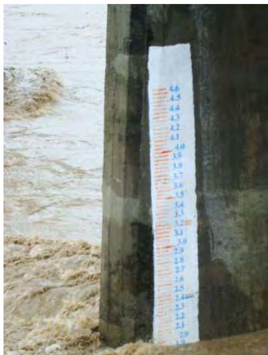
A flood gauge installed by PAGASA in Kabilang-llog Bridge in Boac, Marinduque, to monitor the flood level in Boac, River (Photo by Myke Magalang)
