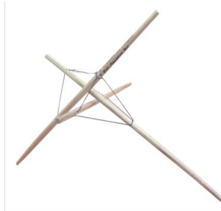
Fig. 4. Nature of Structure basic minimum unit made of chopsticks and silk string by K. Snelson.
