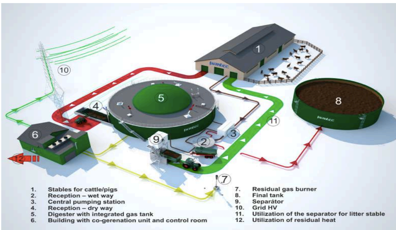
Graph 06: MSMEs network function (exemplified on a project of a Biogas plant; Conel, s.r.o. CZ)
