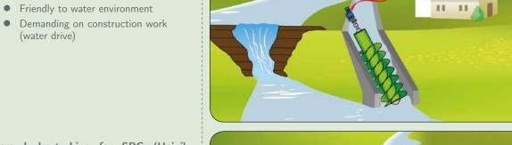
Micro hydro-turbine for SPC (Heinik, Francis, Kaplan,) 5 - 500 kWe; suitable solution for streams and rivers with varying and substantial gradient of water flow
